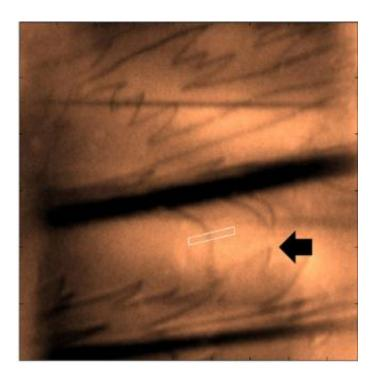
An X-ray reflection interface microscope (XRIM)image of an orthoclase (001) surface. The black arrow indicates a mono-molecular step 0.65 nm in height.
