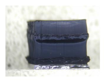
The nanotube array alone on its substrate. Credit: University of Cincinnati
