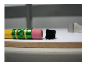
"The harmonious combination of substrate, alloy catalyst and process conditions was found to consistently produce nanotube arrays more than 7 mm long" says Professor Vesselin Shanov, co-director of Smart Materials Nanotechnology Laboratory at the University of Cincinnati (UC).
