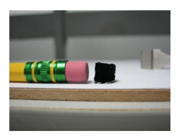
"The harmonious combination of substrate, alloy catalyst and process conditions was found to consistently produce nanotube arrays more than 7 mm long" says Professor Vesselin Shanov, co-director of Smart Materials Nanotechnology Laboratory at the University of Cincinnati (UC).
