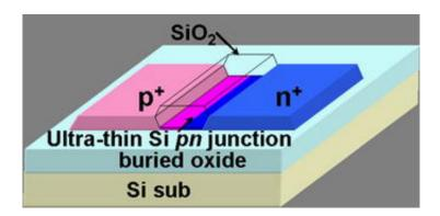
This close-up drawing of the LET shows the ultrathin silicon junction acting as a quantum well. After recombination, the electric carriers are confined into a standing wave, greatly increasing the electroluminescence efficiency. Credit: Shin-ichi Saito, et al.
