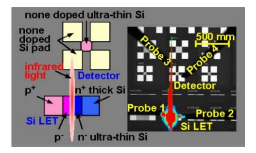
At left, the drawing of the LET describes the scientists' observation, shown in the electroluminescence intensity map at right. The infrared light emitted from
