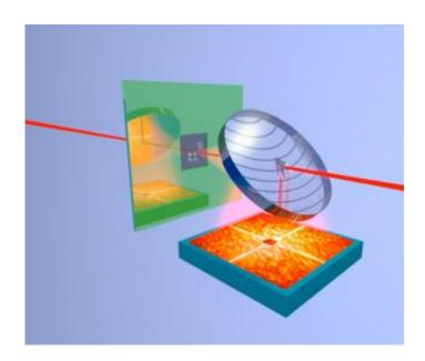
Scematic view of the "flash diffractive imaging" experiment with microstructure samples at the free-electron laser facility FLASH in Hamburg. Credit: H. N. Chapman et al.
