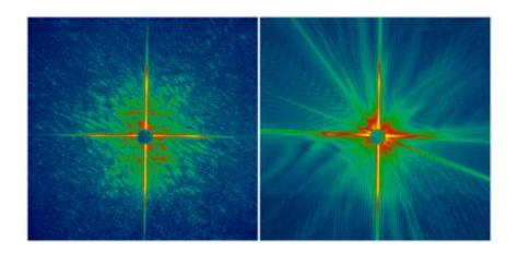
Left: Diffraction image of a microstructure sample taken in an experiment at the free-electron laser facility FLASH in Hamburg using a single ultra-short, extremely intensive and coherent laser shot of just 25 femtoseconds duration. Right: The same sample after its damage by the first laser shot. Credit: H. N. Chapman et al.
