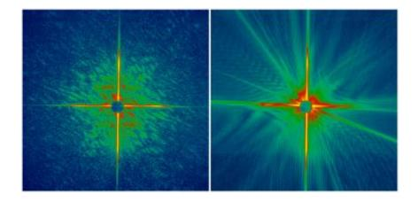
Left: Diffraction image of a microstructure sample taken in an experiment at the free-electron laser facility FLASH in Hamburg using a single ultra-short, extremely intensive and coherent laser shot of just 25 femtoseconds duration. Right: The same sample after its damage by the first laser shot. Credit: H. N. Chapman et al.
