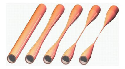
A depiction of the gradual reduction of the diameter of a carbon nanotube via the process created by Yuzvinsky et al. (Image courtesy Tom Yuzvinsky)
