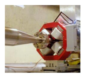
The first bunch compressor for the LCLS, being installed during the current shutdown. This quadrupole magnet is situated on the downstream end of the bunch compressor nearest the electron gun.
