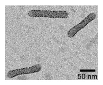
This electron microscope image clearly shows the tightly packed cylinders of gold nanoparticles. Credit: Eugene Zubarev/Rice University
