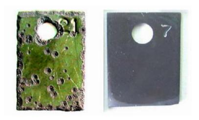
This macrophotograph compares commercial nickel-based Alloy 600 (top) and Argonne&acutes new alloy after 5,700 hours of exposure to the same metal-dusting environment at 593°C.
