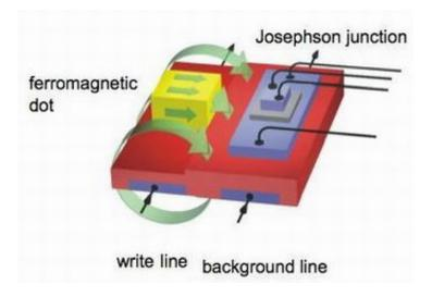
Schematic drawing of a single superconducting memory cell.
