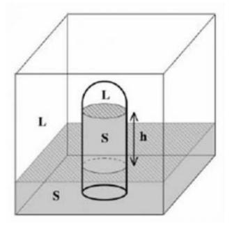
Solid helium [S] comes to a higher level inside the tube than outside. Liquid helium [L] fills the rest of the apparatus. The height difference [h] can be eliminated only if liquid helium can pass through the solid helium blocking the tube. Credit: Image: Frederic Caupin
