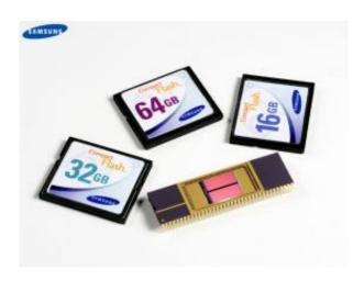
Samsung Electronics today announced that it has developed the industry's first 40-nanometer memory device. The new 32 Gigabit (Gb) NAND flash device is the first memory to incorporate a Charge Trap Flash (CTF) architecture, a revolutionary new approach to further increase manufacturing efficiency while greatly improving performance.
