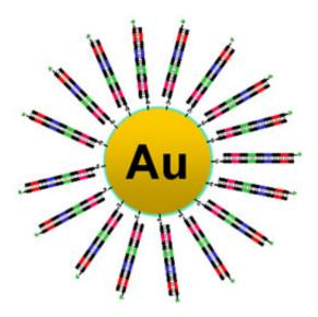
By attaching DNA strands to gold nanoparticles, Berkeley Lab and UC Berkeley scientists have developed a ruler capable of measuring protein-DNA interactions.
