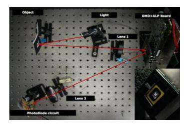
DMDs, which are fabricated by Texas Instruments and today used primarily in digital televisions and projectors, are devices capable of converting digital information to light and vice versa. Built on a microchip chassis, a DMD is covered with tiny mirrors, each about the size of a microbe, that are capable of facing only two directions. They appear bright when facing one way and dark when facing the other, so when a computer views them, it sees them as 1's or 0's.
