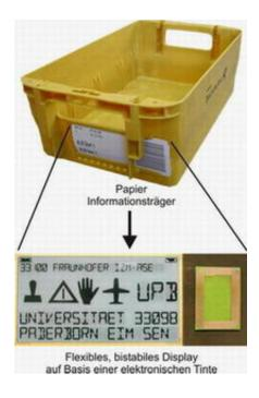
Flexible, bistable display based on electronic ink (passive D-RFID). © Viossloh IT
