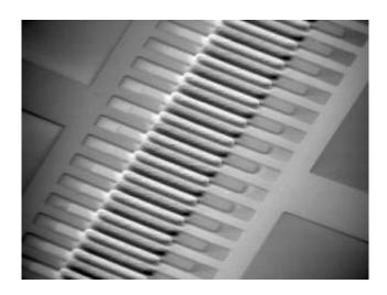
This micropump developed by MIT researchers allows high speed flows through microchannels with an input of only a few volts of electricity, making it possible to create portable "lab on a chip" devices. The three-dimensional, alternating current electro-osmotic pump consists of interdigitated stepped gold microelectrodes on a glass substrate. Credit: J.P. Urbanski
