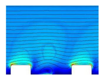
This simulation of three-dimensional alternating current electro-osmosis shows liquid flowing around stepped electrodes. The "fluid conveyor belt" allows fluid to be rapidly pumped through microchannels. Credit: Martin Bazant
