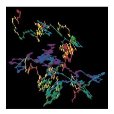
Twenty seconds of a measured random walk trajectory for a micrometer-sized ellipsoid undergoing Brownian motion in water. The ellipsoid orientation, labeled with rainbow colors, illustrates the coupling of orientation and displacement and shows clearly that the ellipsoid diffuses faster along its long axis compared to its short axis.
