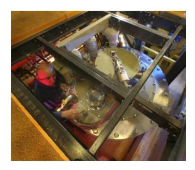
Dwight Rickel of the National High Magnetic Field Laboratory's Pulsed Field Facility (NHMFL-PFF) at Los Alamos National Laboratory checks the 100 Tesla Multi-shot Magnet. Recently commissioned for user operation at 85 tesla, the magnet opens up new frontiers for scientific research. Credit: LeRoy N. Sanchez
