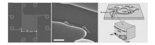
The scanning electron micrograph at left shows an overview of the silicon track, designed to coax the bacteria into moving in a uniform direction around the circular tracks. In the center, two cells glide along the wall in the track. The illustration at right of a circular track shows how the bacteria bind to and pull the rotor. Image credit: Yuichi Hiratsuka, et al.
