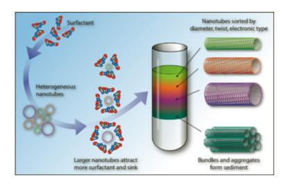
Single-walled carbon nanotubes are coated in soap-like molecules called surfactants, then spun at tens of thousands of rotations per minute in an ultracentrifuge. The resulting density gradient sorts the nanotubes according to diameter, twist and electronic structure. Credit: Zina Deretsky (adapted from Arnold et al.), NSF
