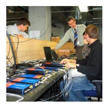
Satellite navigation receivers under test at Septentrio. Credits: ESA / Septentrio Satellite Navigation NV
