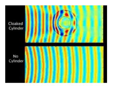
A team led by scientists at Duke University's Pratt School of Engineering has demonstrated the first working "invisibility cloak." The cloak deflects microwave beams so they flow around a "hidden" object inside with little distortion, making it appear almost as if nothing were there at all.
