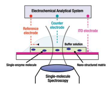
PNNL researchers are developing a new approach for studying the molecular mechanisms of enzymes. They use a three-electrode platform to oxidize and reduce enzymes, then capture chemical reaction data with a single molecule spectroscope.
