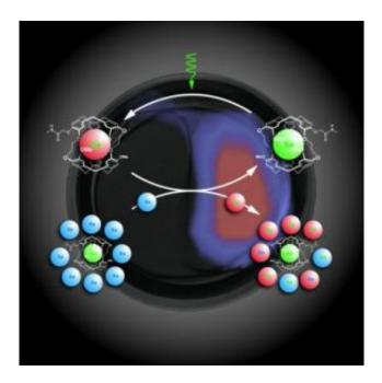
HYPER-CEST is a technique for enhancing the signal of molecular MRI through the combination of hyperpoalized xenon and the CEST technlogy. Credit: Lawrence Berkeley National Laboratory
