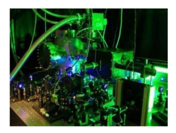
JILA's scanning photoionization microscope (SPIM) includes an optical microscope (in vacuum chamber, background) and an ultrafast laser (appears as blue, foreground). Credit: Credit: O.L.A. Monti, T.A. Baker, and D.J. Nesbitt/JILA
