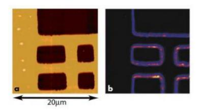
A false color SPIM image (b) reveals the same physical structure of a gold pattern on glass as an atomic force microscope image (a), but the high intensity regions in the SPIM image indicate that electron ejection is much more efficient at metal edge discontinuities. Credit: Credit: O.L.A. Monti, T.A. Baker, and D.J. Nesbitt/JILA
