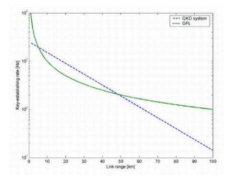
This graph compares the speed it takes for establishing secret keys in a both a quantum key distribution system and the new giant fiber laser system. As the distance increases to more than 48 km, the classical laser system demonstrates its advantages, especially at longer distances. Credit: Scheuer and Yariv.
