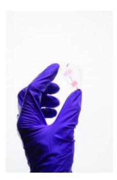
A microfluidic chip. Microfluidics is the science of manipulating fluids on the micron scale, a unit of measurement much narrower than the diameter of a human hair. Credit: Photo by Peter Kiar
