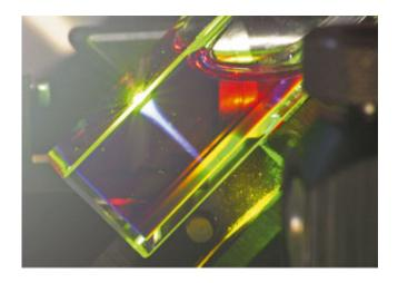
Experiment to show the changes in the wave length. The green light directed into the solution reappears as blue light after it has been converted. Image: Max Planck Institute for Polymer Research
