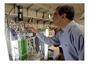
Himadri Pakrasi explains the photobioreactor in his Rebstock Hall laboratory. Inside the tube photosynthetic bacteria are making ethanol more efficiently than other forms of biomass because the ccyanobacteria are natural fermentators. Photo by David Kilper / WUSTL Photo
