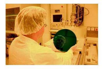
The 300-mm wafers are coated with an etch-resistant film in the cleanroom. Currently being tested: Masks made of aluminum nitride instead of silicon dioxide. © Fraunhofer IKTS
