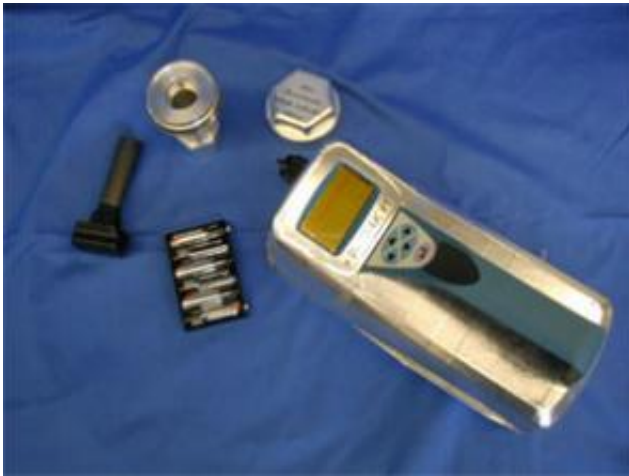
Photo of the P-Trak air quality measurement device made by TSI. Credit: NASA
