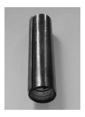
The display coiled up into a self-locking tube.
