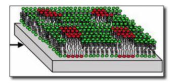
Researchers induced the formation of tiny lipid raft-like gel domains on silicon chips (above). They then used LLNL's high-resolution secondary ion mass spectrometer, the NanoSIMS, to image the samples and detect the gel domains at lateral dimensions as small as 100 nanometers (about 1,000 times smaller than the diameter of a human hair). The gel domains are shown as red in both the schematic and the NanoSIMS ion image (below). Credit: Lawrence Livermore National Laboratory
