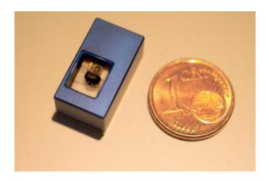
This projector gets by with a single mirror instead of a million. As a result, it is small and easily manageable. © Fraunhofer IOF
