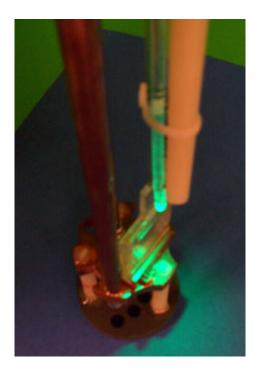
A high-powered electromagnet allowed researchers to increase, eliminate and even decrease the effects of gravity on live paramecia in a vial of pond water. (The paramecia swim harder when gravity increases.) Methods for studying a biological response to altered gravity had been few and troublesome in Earthbased laboratories. Image: Karine Guevorkian and James Valles
