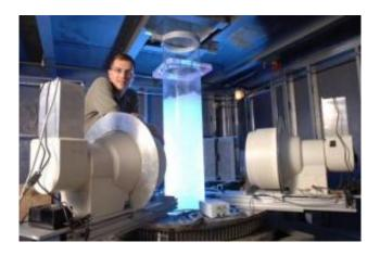
Ted Heindel will use Iowa State's X-ray flow visualization facility to observe and measure the action inside a fluidized bed where biomass can be converted into flammable gases. Credit: Photo by Bob Elbert/Iowa State University
