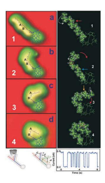
Scientists used a scanning tunneling microscope to manipulate chlorophyll-a into four positions. Art by: Saw-Wai Hla
