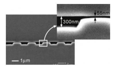
This scanning electron microscopy (SEM) image shows MIT's new nanoscale molecular sieve, which consists of thousands of alternating deep (300 nanometers or billionths of a meter) and shallow (55 nanometers) regions. The deep and shallow regions act together to form energy barriers that separate proteins by size. Pores of different sizes can be engineered for different filters to capture specific proteins. Image courtesy / Han lab
