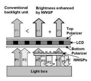
On the left side of this drawing, P1 light is transmitted through the LCD panel, while a conventional bottom polarizer absorbs P2 light. On the right, the scientists' new nano-wire grid polarizer recycles some of the otherwise-absorbed P2 light back to the light box, where it is partially converted to P1, and the process repeats. Image credit: Sang Hoon Kim et al.
