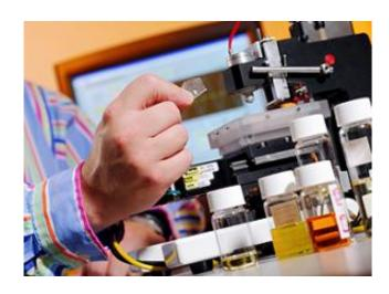
Georgia Tech Associate Professor Carson Meredith and graduate student Pedro Zapata developed this combinatorial fuel cell membrane using a high-throughput conductivity instrument. Georgia Tech Photo: Gary Meek
