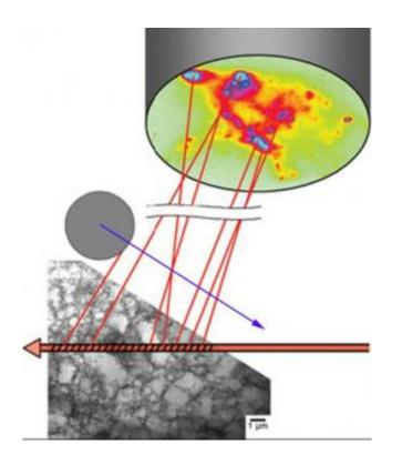
Novel 3-D microbeam experiment enables direct proof of the Mughrabi model of metal stress. Submicron X-ray beam (broad arrow) penetrates a deformed copper single crystal and is diffracted onto a CCD detector. Platinum wire profiler (circle) traverses the sample and successively intercepts diffracted Xrays, providing depth measurement and allowing strains to be measured from individual dislocation cells. Credit: NIST
