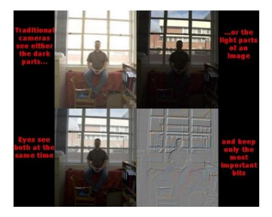
This image shows how our eyes work versus how cameras work.
