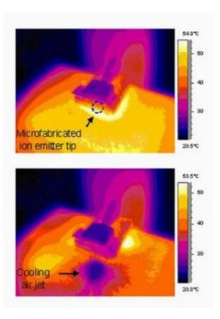
Infrared images show how a new UW micro-pump cools a heated surface: (Top) The air pump is off. (Bottom) The air pump is on. Credit: University of Washington
