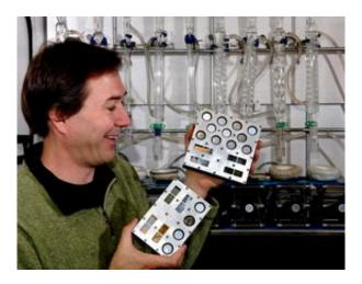
Mat Celina displays the piezoelectric polymer films that will be tested on an upcoming Materials International Space Station Experiment. (Photo by Randy Montoya)
