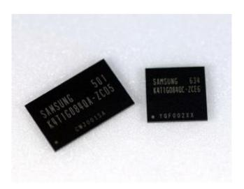
Samsung Electronics, the world leader in advanced memory technology, announced today mass production of 1Gigabit (Gb) DDR2 DRAM memory using 80 nanometer (nm) process technology. While monolithic 1Gb DDR2 is available today, it is produced with more costly and less efficient 90 nm technology.
