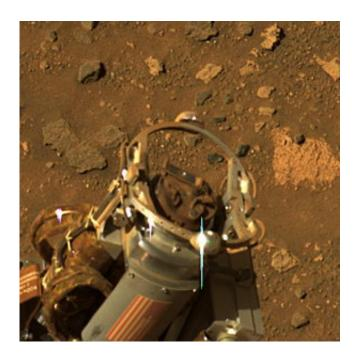
An abundance of iron oxide minerals in Martian dust have given Spirit&acutes robotic arm and rock abrasion tool a reddish-brown veneer. Image credit:
