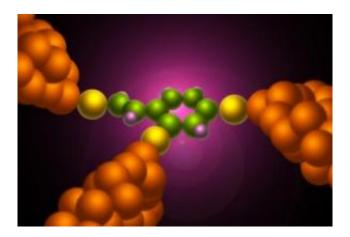
Artist's conception of a Quantum Interference Effect Transistor (QuIET). The colored spheres represent individual carbon (green), hydrogen (purple), and sulfur (yellow) atoms, while the three gold structures represent the metallic contacts. A voltage applied to the leftmost contact regulates the flow of current between the other two. (IMAGE: ACS Nano Letters)
