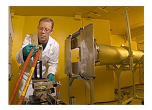
NIST scientist David Jacobson prepares an experimental fuel cell for real-time imaging at the NIST Center for Neutron Research. A new research station at the center produces still images akin to CAT scans and movies recorded at a rate of up to 30 frames per second, or 30 times faster than a first-generation instrument. ©Robert Rathe
