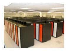
Oak Ridge National Laboratory has increased computing power of its Cray supercomputing system (shown here) to 54 teraflops, or 54 trillion mathematical calculations per second, placing it among the most powerful open scientific systems in the world.
