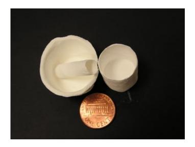
Further, the material can be cast into different three-dimensional shapes, with different functions. The researchers have created tubes, bowls and cups using this process. These three-dimensional hollow objects can be manipulated by hand and trimmed with scissors, the researchers report.
