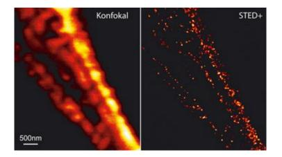
A look at the inside of cells becomes sharper: Both figures above show the filaments in a human nerve cell; left with a common confocal microscope, right with a STED microscope plus mathematical deconvolution. The resolution of the STED microscope is better by more than an order of magnitude. Image: MPI für biophysikalische Chemie
